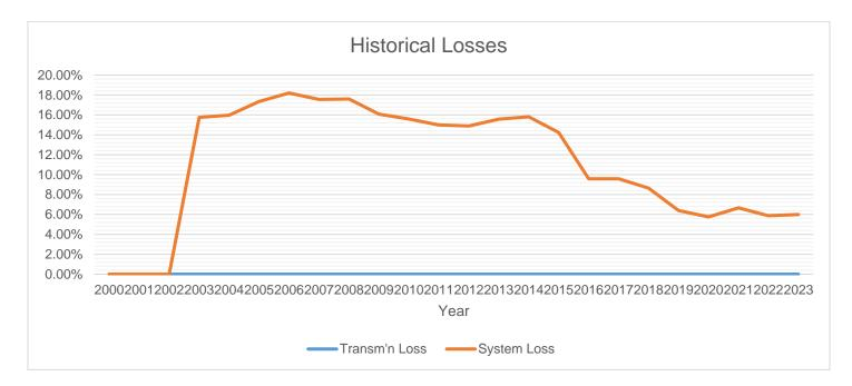
Historically, System Loss ranged from 5.75% to 18.20%. System Loss registered high at 18.20% on year 2006 because at that time, electric distribution system going to Panukulan, Quezon is only single phase with undersized conductors resulting to low voltage and unbalanced system. Also, there was ongoing electrification to different barangays of Polillo, Panukulan, and Burdeos resulted to additional line losses for Polillo Island Electric Distribution System.
